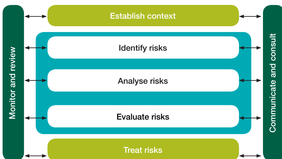
Figure 4.1: Components of a risk management framework – reproduced from Australian/New Zealand Risk Management Standard AS/NZS 4360:2004
